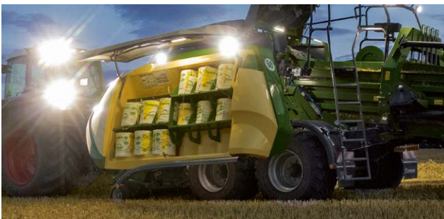
Lights inside the twine boxes
